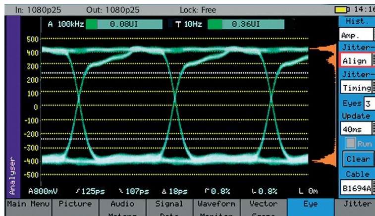
PHABRIX Sx E eye and Jitter with automatic measurements at SD-SDI, HD-SDI, 3G-SDI
